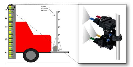
Figure 2. Tower sprayer with detail of mounted Lechler VarioSelect<sup>®</sup> unit.
