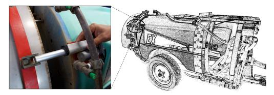
Figure 1. Louvre system mounted on conventional axial-fan sprayer.
